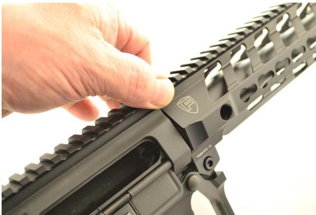
5. Align the top Picatinny rail with the top rail on your upper receiver. (see photo to the left)
